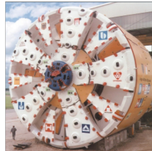
German Tunnel Boring Machine – 46 feet in diameter
